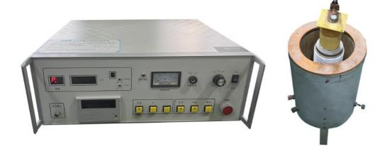
More than "Pass/Fail", the purpose to check the integrity of the vacuum interrupter should include to estimate its lifespan based on its leakage rate.
